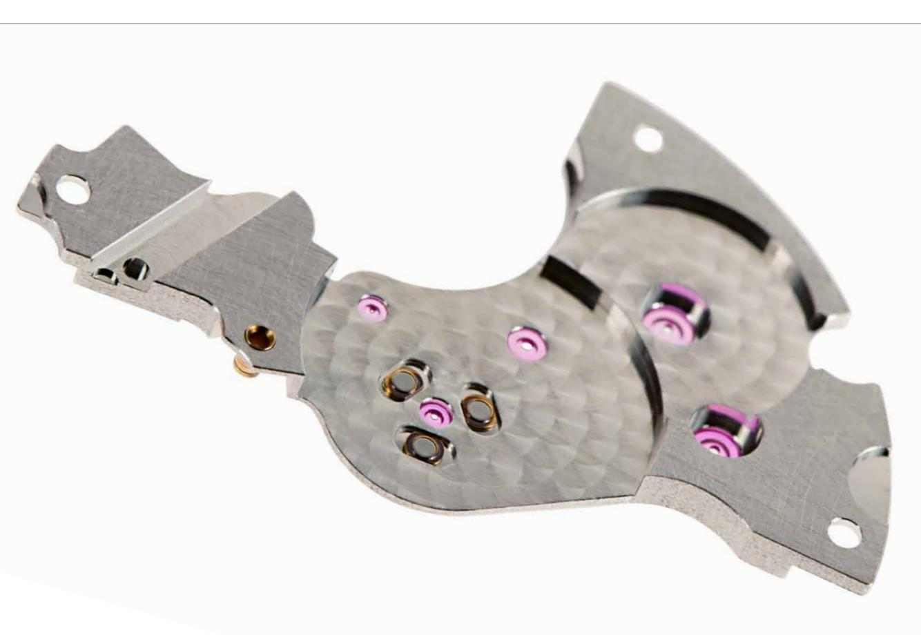
The train bridge removed, showing the gear train with direct seconds drive, (the escape wheel is leaning forwards out of mesh with the centre wheel).
